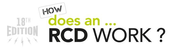
An RCD protects by constantly monitoring the current flowing in the Line/ Phase and Neutral wires supplying a circuit or an individual item of equipment. Under normal circumstances, the current flowing in the two wires is equal. When an earth leakage occurs due to a fault in the circuit or an accident with the equipment, an imbalance occurs, and this is detected by the RCD, which automatically cuts off the power before injury or damage can result
